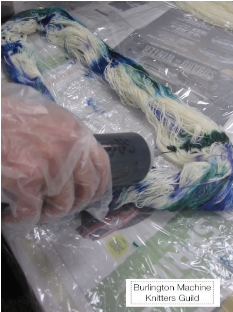
Acid dyes are applied and then blended into the fibres by hand.
